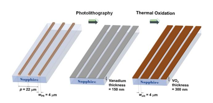
Schematics of fabrication steps: A vanadium slit array is patterned on a c-plane sapphire substrate by photolithography. After that, the vanadium slit array is annealed under optimized oxygen pressure and temperature. After the annealing process, the thickness of the film doubled. Credit: UNIST
