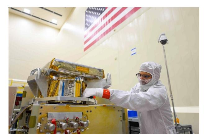
The side of the High-resolution Volatiles and Minerals Moon Mapper (HVM<sup>3</sup>) is seen as the instrument gets unwrapped in a clean room. The JPL-developed imaging spectrometer was later integrated with NASA's Lunar Trailblazer spacecraft. Credit: Lockheed Martin Space
