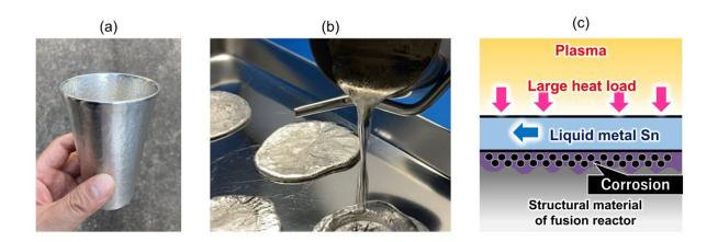
Fig 1. (a) Tin tableware, (b) Liquid metal fluid, (c) Mechanism of liquid metal divertor and corrosion issues. Credit: Masatoshi Kondo
