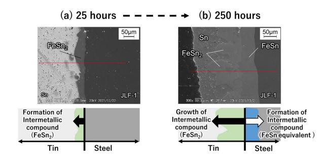
Figure 2. Image of surface layer cross-section of fusion reactor structural material (reduced activation ferritic martensitic steel) immersed in liquid tin. (a) When immersed in liquid tin at 500°C for 25 hours. (b) When immersed in liquid tin at 500°C for 250 hours. Taken using a scanning electron microscope. Credit: Masatoshi Kondo
