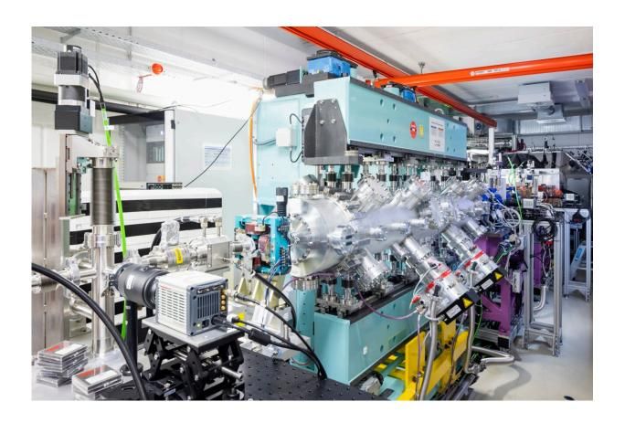
German-French research team builds free-electron laser at the Helmholtz-Zentrum Dresden-Rossendorf (HZDR) driven by particles from a plasma accelerator—and generates well-controllable laser flashes for the first time with this still young technology. In the foreground, the beam line framed by a light-blue magnet arrangement, the undulator; in the background, the metallic beam chamber for the high-power laser DRACO at HZDR. Credit: HZDR/S. Dittrich
