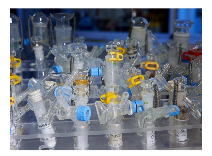
New air- and water-sensitive catalysts are produced and stored in so-called Schlenk vessels under an inert gas atmosphere. Credit: LIKAT/Nordlicht
