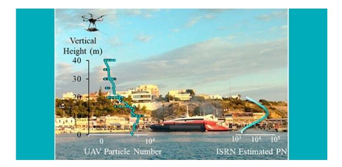
The experimental setup showing UAV (drone) monitoring and improved estimations of particle dispersion from maritime emissions. Credit: Department of Engineering, University of Cambridge
