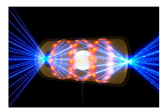
This illustration provided by the National Ignition Facility at the Lawrence Livermore National Laboratory depicts a target pellet inside a hohlraum capsule with laser beams entering through openings on either end. The beams compress and heat the target to the necessary conditions for nuclear fusion to occur. Credit: Lawrence Livermore National Laboratory
