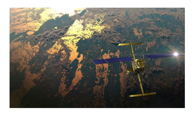
This illustration shows the SWOT satellite in orbit with sunlight glinting off one array of solar panels, as well as both KaRIn instrument antennas deployed. Credit: CNES
