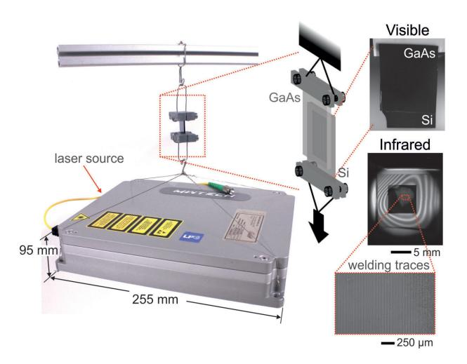
Left: Image of the laser source employed in the experiments hanging in the air by the welding of a silicon (Si) wafer on top of a gallium arsenide (GaAs) one. The unit weighs 3 kg and the welded area is estimated to sustain up to 400 N. Right: Images of the welded pieces taken by means of a visible and an infrared camera, which allows observing the welding pattern in between. Credit: Pol
