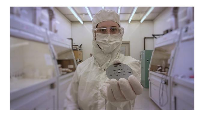
Espenhahn in an HMNTL cleanroom holding a wafer with VCSELs fully integrated on silicon. Credit: The Grainger College of Engineering at University of Illinois Urbana-Champaign
