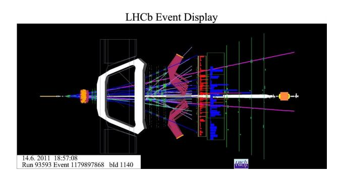
LHCb event display from 2011 showing a B meson decaying into a muon and antimuon pair . Credit: CERN
