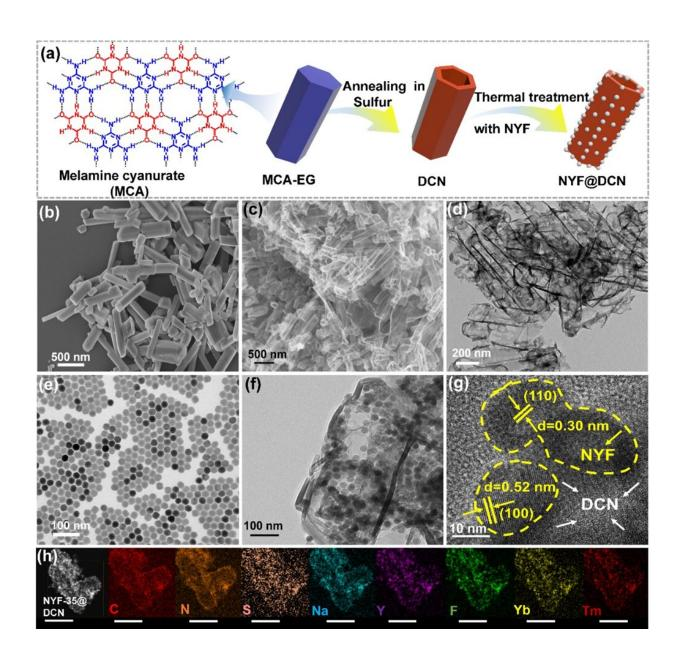
a) Schematic illustration for the fabrication of NYF@DCN. SEM images of b)
