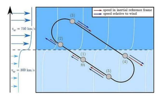
The trajectory of a vehicle performing dynamic soaring in wind shear on the slow and fast solar wind. Credit: *Frontiers in Space Technologies* (2022). DOI: 10.3389/frspt.2022.1017442
