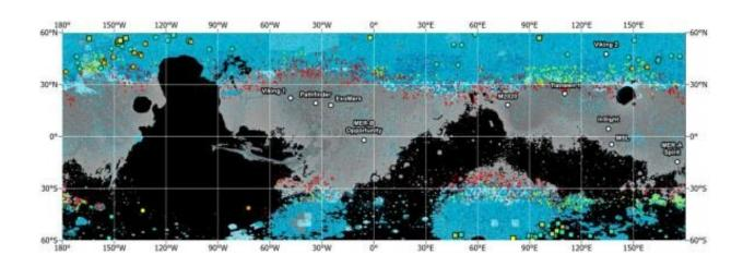
Mars SWIM Project ice consistency results from a depth range of 1–5 m. Map of ice consistency across the study area; blue areas indicate the presence of ice, and red areas contain no ice. A map like this is crucial for planning a landing site with access to water. Credit: NASA
