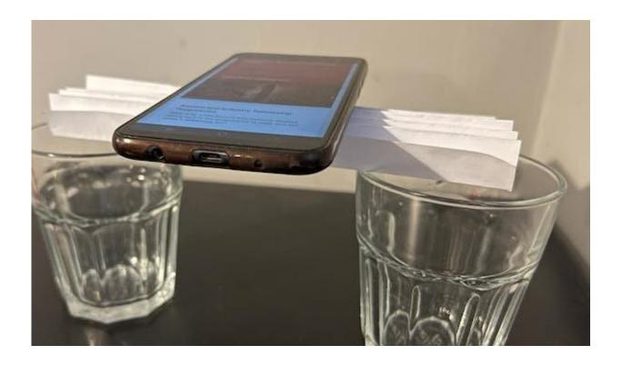
A folded piece of paper in a zig-zag shape could withstand heavy load. Credit: Amin Al-Habaibeh, Author provided.
