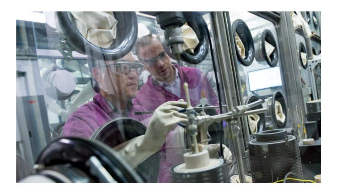
Researchers are searching for the ideal characteristics of molten salt, which can serve as both coolant and fuel in advanced nuclear reactors. Credit: Argonne National Laboratory
