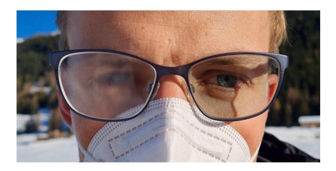
In winter, face masks can lead to fogged glasses. Here, the left lens (right from the reader's perspective) has the new antifogging nanocoating. The other lens is uncoated. Credit: ETH Zurich
