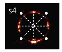
Four defects (d1-d4) in the photonic crystal ring (left) can host a defect photonic crystal mode (e.g., d1) and also fix the orientation of higher-order modes (e.g., s4). Credit: Mingkang Wang and Xiyuan Lu.
