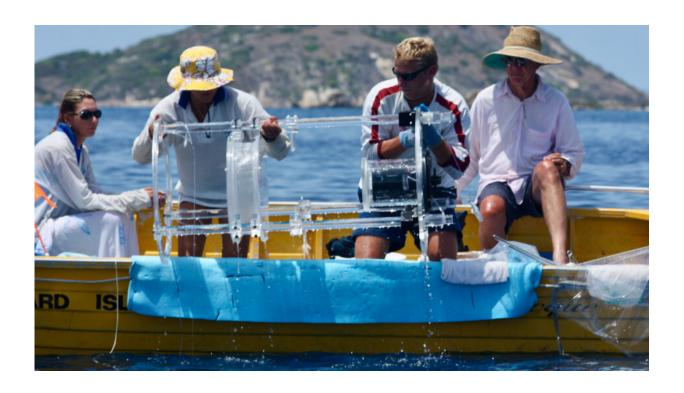
Claire Paris, professor of ocean sciences (center left), and co-author Jean-Olivier Irisson (center right) deploy the Drifting In Situ Chamber (DISC), equipped with an imaging system designed to record larval fish swimming behavior in their natural settings during an expedition at the Australian Museum Lizard Island Research Station. Credit: Lyle Vail
