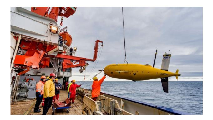
The Autosub Long Range (ALR) autonomous underwater vehicle is deployed in front of the Filchner-Ronne Ice Shelf, where researchers used it to study a warm water current, during an expedition to the Weddell Sea in 2018. Credit: Yannick Kern
