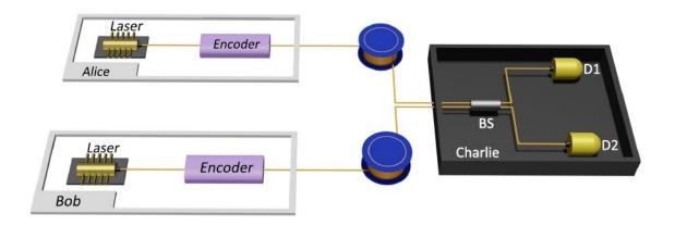
At Alice's (Bob's) site, the simplified transmitter contains a laser source and an encoder. The encoder modulates the phase of the optical pulses. The modulation information of the encoder should be monitored to characterize the deviation between ideal and realistic pulses. If the untrusted Charlie is honest, he measures the signals received using an interference measurement. Credit: Science China Press
