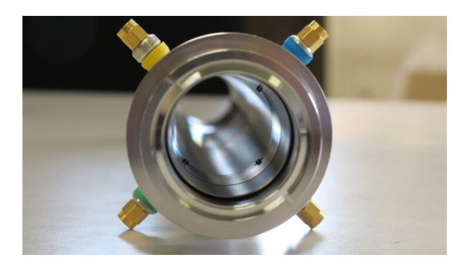
Wideband beam monitor with four rod antennas located at every 90 degrees. Credit: KEK
