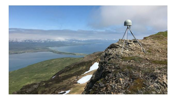
A new algorithm was shown to improve the use of data for earthquake sensing from global navigation satellite system sensors, like this one on the Aleutian Peninsula of Alaska. Credit: Ellie Boyce/UNAVCO, CC BY 4.0
