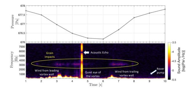
This is a spectrogram of the microphone sound pressure level showing the low frequency wind noise, the high frequency grain impacts and also the rover pump harmonic at 760 Hz. A large grain impact causes an acoustic echo at approximately 6 kHz due to sound reflections from the base of the microphone. Credit: N. Murdoch / ISAE-SUPAERO
