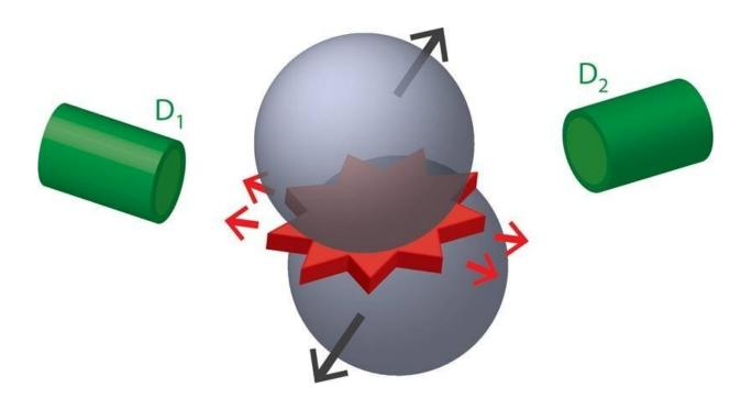
Optical deblurring, applied to measurements of nuclear collisions, can reveal what detectors (D1 and D2) would see if they were optimally oriented relative to the initial geometry of the collisions. Credit: Pawel Danielewicz, Michigan State University
