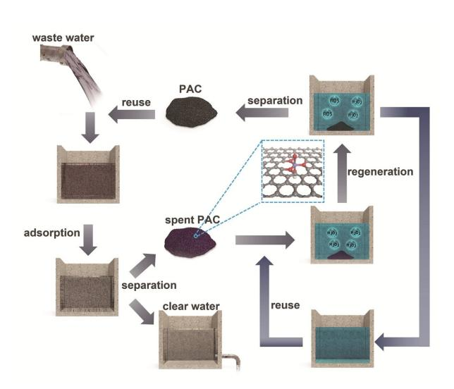
The H2O2-based PAC adsorption/regeneration process for wastewater treatment. Credit: NIMTE
