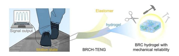
The breakage-resistant conductive hydrogel and its potential application in mechanical-reliable TENG. Credit: NIMTE
