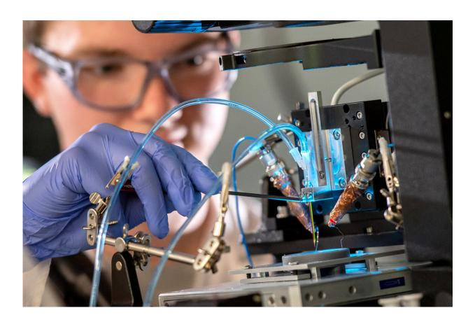
A very special kind of 3D printer: Masters student Simon Sprengel makes some final adjustments to allow two metal solutions to flow simultaneously through the tiny printing nozzle. Credit: University of Oldenburg
