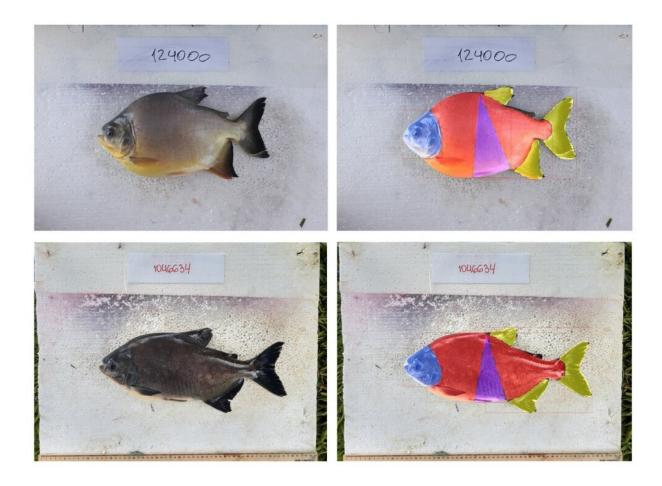
Software developed by Brazilians automatically measures pacus using artificial intelligence. Specimens with round body (top) and elliptical body. On the right, parts selected by the program via machine learning. Credit: Diogo Hashimoto/UNESP
