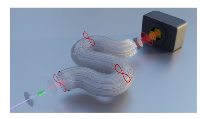
Schematic overview of a phase-separated Anderson localization fiber as quantum channel between a transmitter and receiver. The illustration shows that quantum correlations such as entanglement are maintained during transport from the transmitter (generation) to receiver (detection) all the way along the fiber. Credit: ICFO/ A. Cuevas
