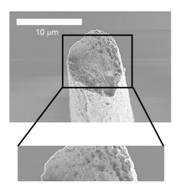
A highly magnified view of a cross section of a CNF. Credit: *Nano Letters* (2022). DOI: 10.1021/acs.nanolett.2c02057
