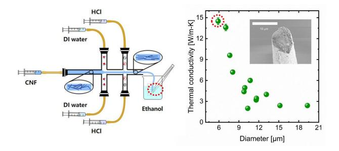
Flow focusing and CNF. The apparatus to create thermally conducting CNF using disorganized CNF, water and hydrochloric acid (left). A graph showing how thermal conductivity of the sample changes with its diameter. (right). Credit: *Nano Letters* (2022). DOI: 10.1021/acs.nanolett.2c02057
