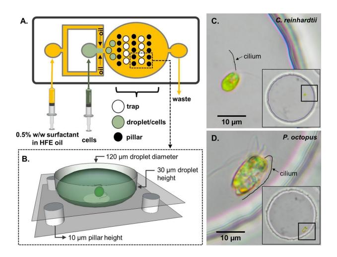
Schematic of the experimental set-up. (**A**) A two-layer microfluidic device with embedded single-cell traps, and syringes used for perfusion of the carrier oil phase and an aqueous suspension containing live motile cells. (**B**) 3D rendering of a single trap in which a cell can be stably trapped and imaged for hours. To demonstrate variability in swimming behavior, we studied two species of motile algae, images show respectively: (**C**) a single *Chlamydomonas reinhardtii* (CR)
