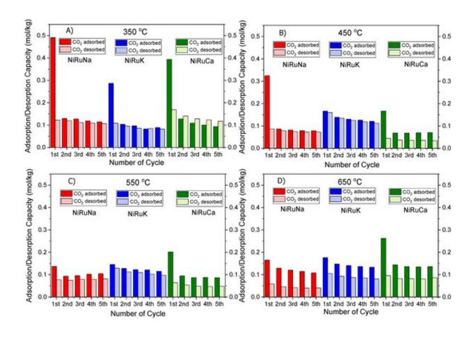
CO2 Adsorption/desorption cycles of NiRuNa, NiRuK and NiRuCa at (A) 350 °C, (B) 450 °C, (C) 550 °C and (D) 650 °C. Credit: *Nanoscale* (2022). DOI: 10.1039/D2NR02688K
