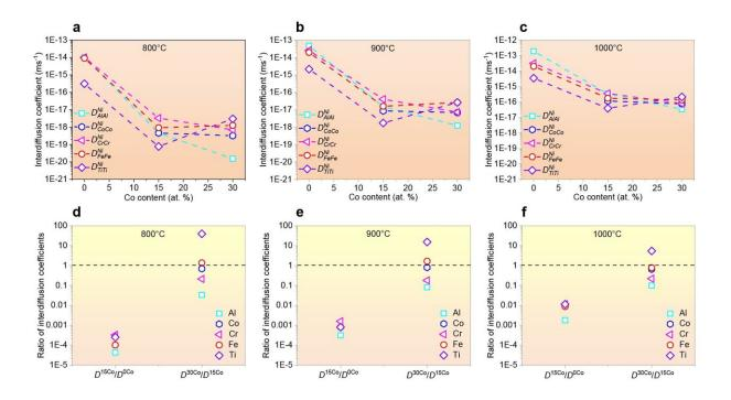
Calculated main interdiffusion coefficients of aluminium (Al), cobalt (Co), chromium (Cr), iron (Fe), and titanium (Ti) elements in the Ni59.9-xCoxFe13Cr15Al6Ti6B0.1 (at.%) alloy. a–c 800 °C, 900 °C, and 1000 °C. d–f The variations of the ratio of interdiffusion coefficients by increasing the cobalt content at 800 °C, 900 °C, and 1000 °C. Credit: Xiao, B. et al, *Nature Communications* (2022). DOI: 10.1038/s41467-022-32620-6
