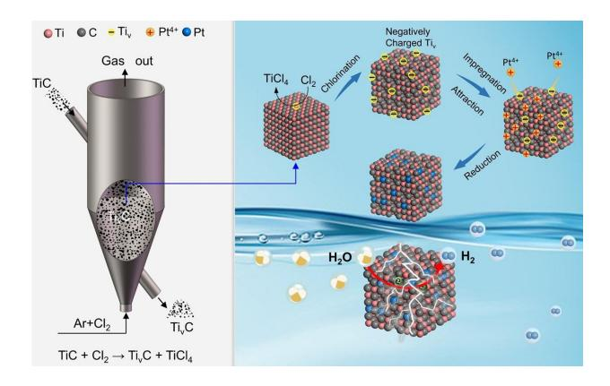
Schematic diagram of the cation defect engineering fluidized technique. Credit: Xiang Maoqiao
