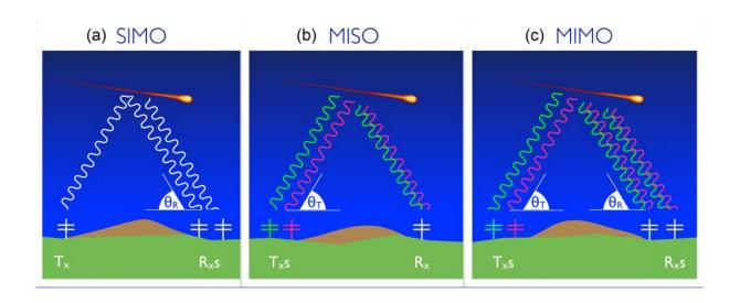
A diagram of different radar systems that can be used to detect ion trails, such as those produced by meteors. SIMO, (a single transmitter and an interferometric receiver), MISO (multiple transmitters and a single receiver) and MIMO (multiple transmitters and receivers). Credit: *Atmospheric Measurement Techniques* (2019). DOI: 10.5194/amt-12-2113-2019
