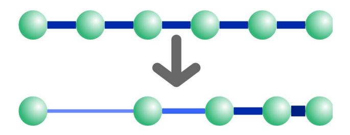
To make a synthetic black hole, just take a chain of atoms (green), and change how easy it is for an electron to jump between each atomic site, represented here by the colour and width of the blue interatomic bonds. The varied bond strength in the lower chain mimics the warping of spacetime in the presence of a black hole. This way, the incredible physics of black holes can be explored in a lab on Earth. Credit: University of Amsterdam
