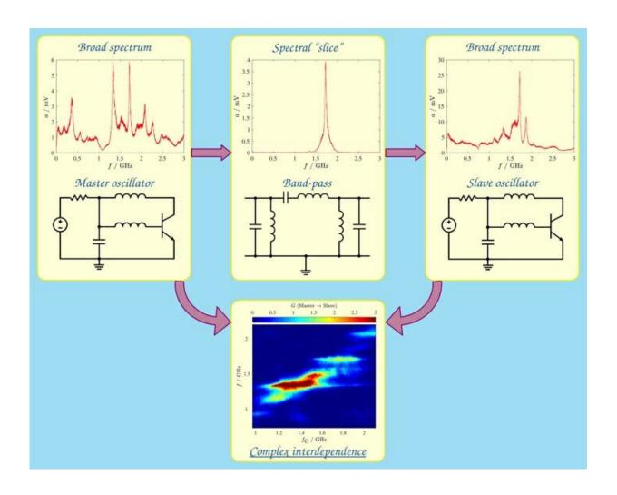
Conceptual overview of the coupling scheme between a master and a slave chaotic oscillator via a band-pass filter, and the resulting complex interdependence between their activities. Credit: *Chaos, Solitons & Fractals* (2022). DOI: 10.1016/j.chaos.2022.112854
