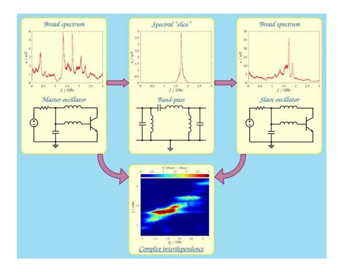
Conceptual overview of the coupling scheme between a master and a slave chaotic oscillator via a band-pass filter, and the resulting complex interdependence between their activities. Credit: *Chaos, Solitons & Fractals* (2022). DOI: 10.1016/j.chaos.2022.112854
