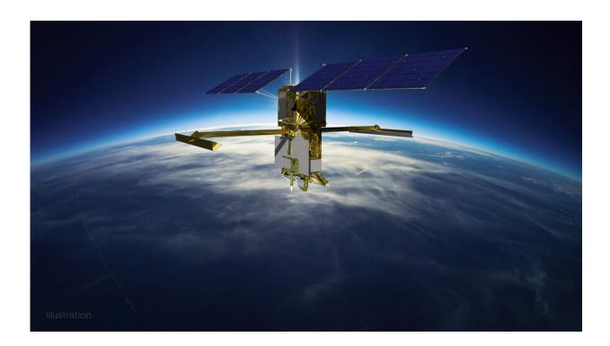
This illustration shows the Surface Water and Ocean Topography (SWOT) satellite in orbit with its solar panels and KaRIn instrument antennas deployed. Credit: CNES
