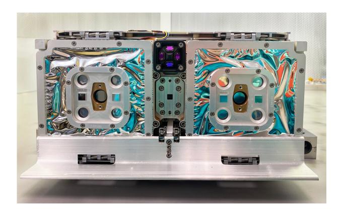
The CTIM detector from a different angle. The metal shelf attached to the bottom front is not part of the device. Credit: Tim Hellickson, LASP
