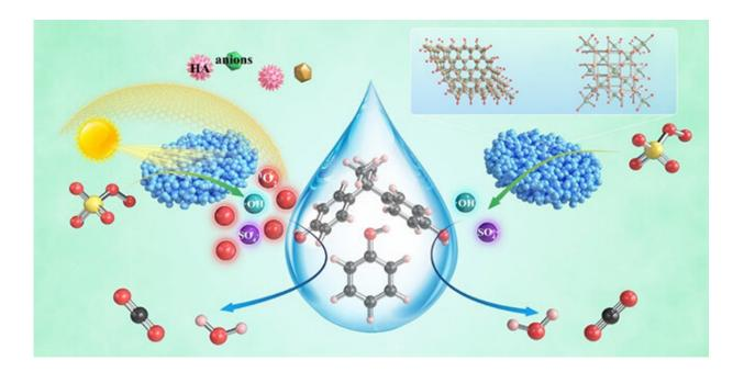
Possible mechanisms of organic pollutant degradation in ZFO-4/PMS/vis system (left) and ZFO-4/PMS system. Credit: Zhang Liang
