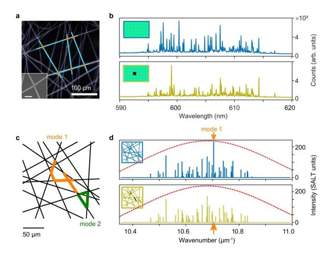
Spectral sensitivity of network lasers to pump profile. a Fluorescence image of a photonic network with interconnected dye-doped polymer nanofibers. As a guide to the eye, we highlight the graph topology (edges as blue lines, nodes as orange dots) over a few links as an example. Inset: scanning electron microscopy image of a node of the network formed by annealing two nanofibers (scale bar =  $1 \mu m$ ).
