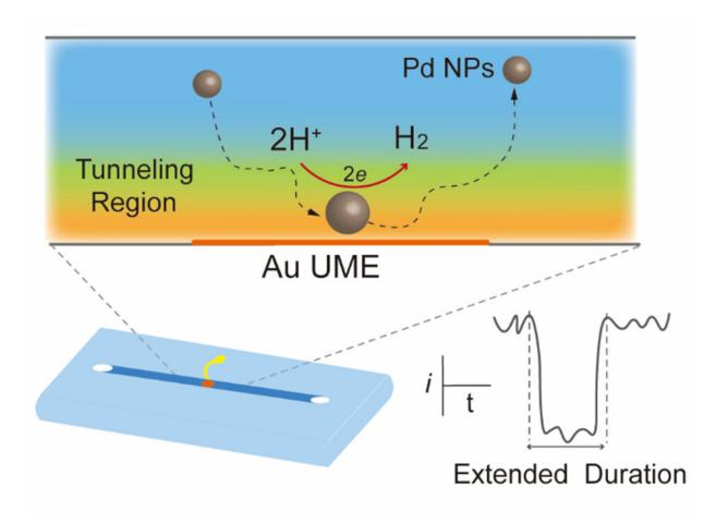
The short collision duration of single nanoparticles hinders the further improvement in their electrocatalytic performance. Here, to increase the collision duration of single nanoparticles in the electron tunneling region, enhanced near-wall hindered diffusion is introduced in the stochastic collision
