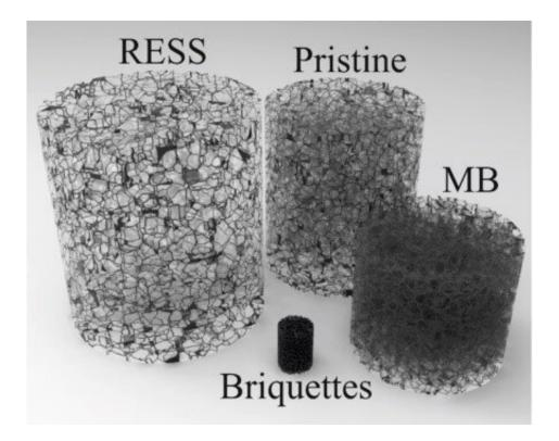
Illustrative representation of the bulk density difference between the four kinds of single-walled carbon nanotubes used, from the left: RESS (expanded), pristine, briquette (compressed), and commercial masterbatch (MB). The cylinders are of equal mass. Credit: Hassaan Butt et al./Carbon.
