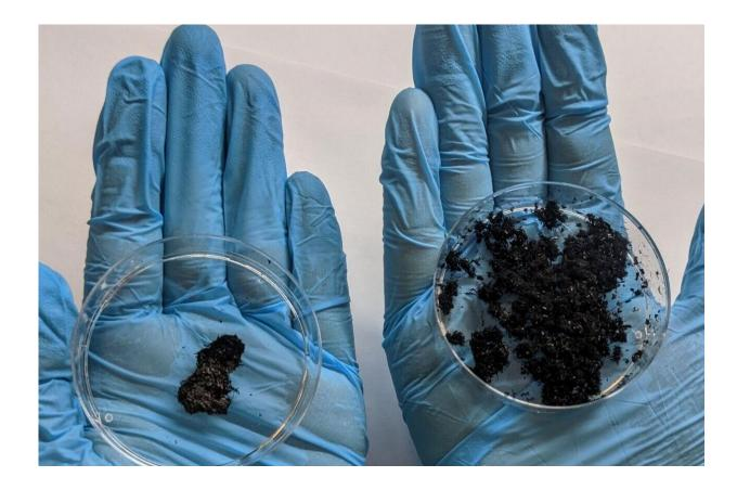
Compressed and expanded carbon nanotube powder for polymer composite manufacture. The study showed the resulting composite material quality to be the same, regardless of which powder was used. That said, the dense powder is more convenient in production. Credit: Hassaan Butt/Skoltech.
