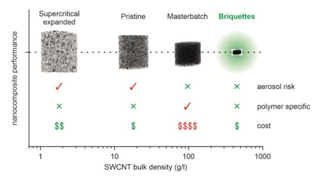
Advantages of the use of briquette-packed carbon nanotubes for manufacturing polymer nanocomposites over the available alternatives. Credit: Hassaan Butt et al./Carbon.
