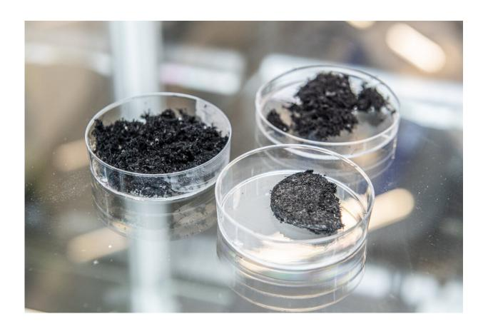
Carbon nanotube powders of varying density for polymer nanocomposite manufacture. The study showed the resulting composite material quality to be the same, regardless of which powder is used. That said, denser powder is more convenient in production. Credit: Timur Sabirov/Skoltech.
