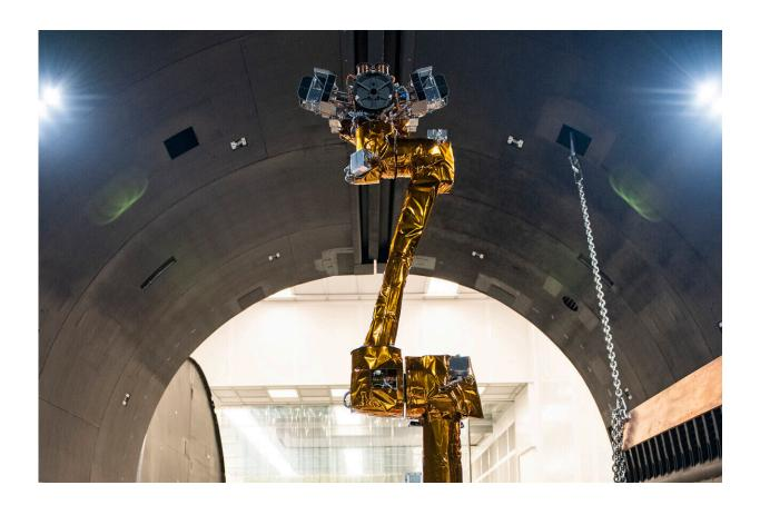
Members of the U.S. Naval Research Laboratory's Robotic Servicing of Geosynchronous Satellites (RSGS) team prepare flight Robotic Arm System (RAS) #1 for thermal vacuum (TVAC) testing in Washington, D.C. June 16, 2022. TVAC testing exposes flight hardware to a vacuum environment and cycles over a wide range of temperatures to ensure the hardware will survive the harsh environment of space. Credit: U.S. Navy/Sarah Peterson
