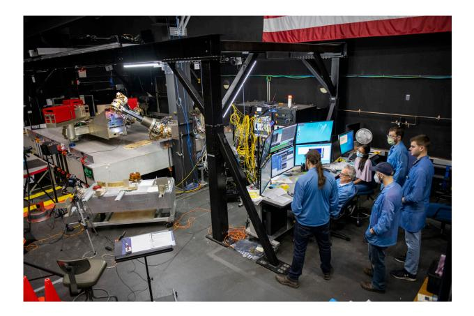
The U.S. Naval Research Laboratory's Robotic Servicing of Geosynchronous Satellites (RSGS) Integration and Test team analyzes data collected from contact dynamic testing on the robotic test bed in Washington, D.C. June 16, 2022. Contact dynamic testing allows the team to charaterize how the payload will behave when servicing client spacecraft. Credit: U.S. Navy/Sarah Peterson
