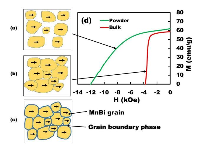
(a) Shows the magnetic MnBi particles/grains separately in the powder. (b)Shows the "bulk" version, where the particles/grains are now touching because of the process of forming the magnet without any added grain boundary materials.(c) Shows the MnBi grains coated with the grain boundary material, illustrating how the grains are no longer touching. The graph illustrates the demagnetization of the magnet in the bulk and powder phases. Credit: U.S. Department of Energy
