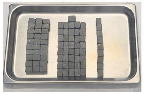
This image shows the smaller and larger magnets constructed in the lab, demonstrating how the process is upscaled. Credit: U.S. Department of Energy Ames National Laboratory
