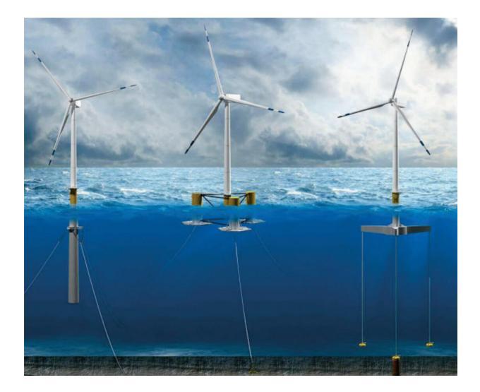
Deep-water sites require floating offshore wind technology, with turbines mounted to a floating foundation or platform that is anchored to the seabed with
