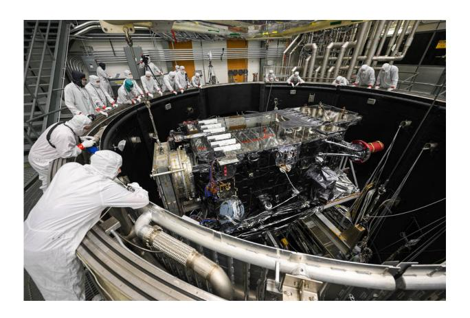
GOES-U is lowered into the thermal vacuum chamber. Credit: Lockheed Martin
