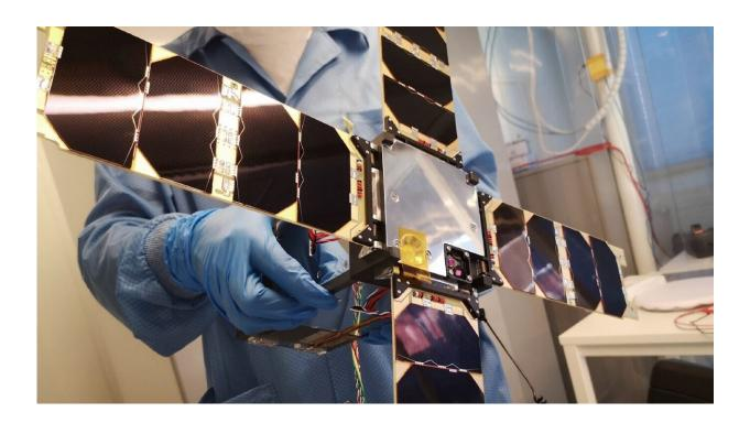
The 2-unit Sunstorm CubeSat carries the X-ray Flux Monitor, used to monitor Xray flares associated with coronal mass ejections, a major driver of space weather. The XFM aperture can be seen in the black lower right corner of the front of the CubeSat as oriented towards the viewer. Credit: Kuva Space
