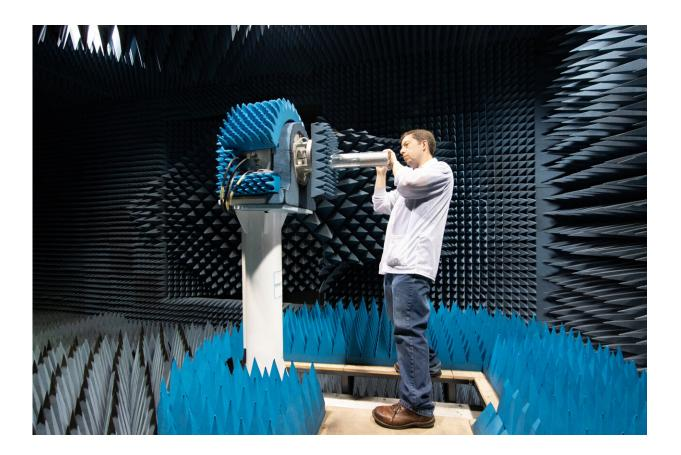
Mechanical Engineer Josh Yacobucci prepares to test a sounding rocket subpayload cannister in the anechoic chamber at NASA's Wallops Flight Facility near Chincoteague, Virginia. Credit: NASA's Wallops Flight Facility/Berit Bland
